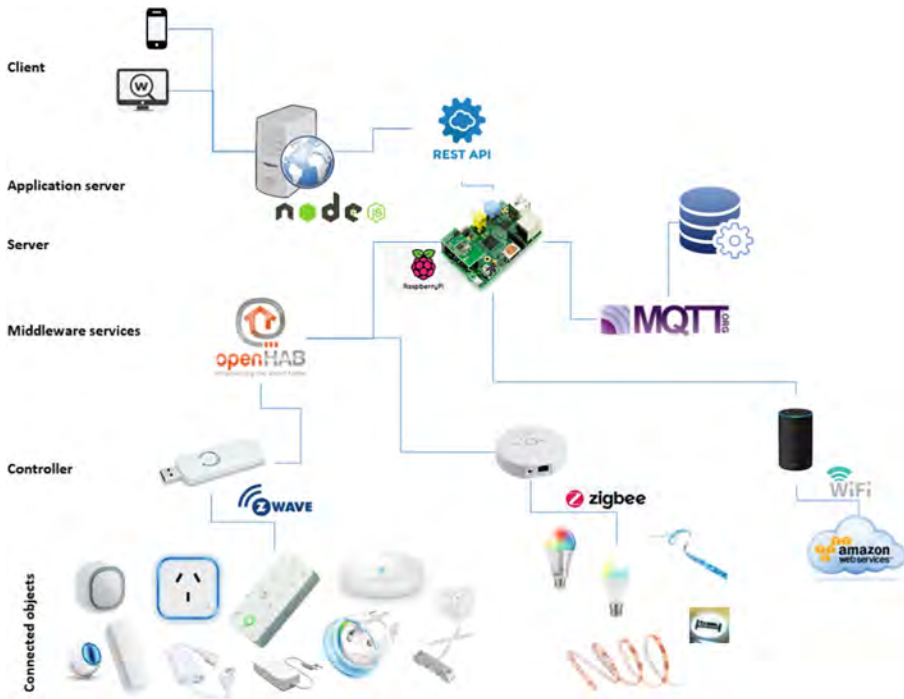
Fig. 2. Physical architecture of the IoT components for AAL system design.
